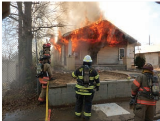
Flashover, from research in South Carolina.
