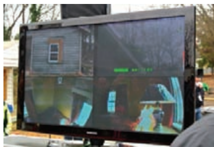
The screen in the photo shows the NIST cameras inside and outside the house as the fire grows and the fire sprinkler activates.
